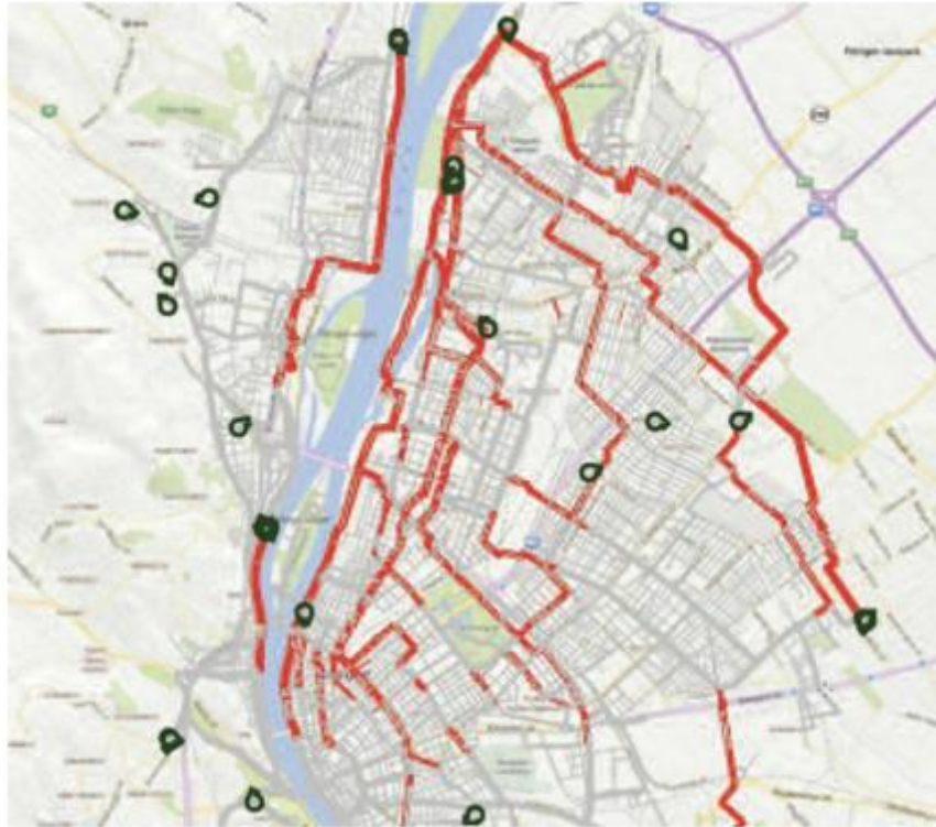
Pipes sections in Budapest District marked in red where the minimum water speed exceeds 0.2 m/s in the main pipes
