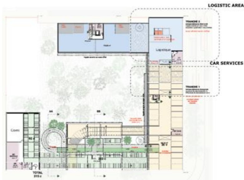
Figure 8 - Detail of the underground space in which the Micro Hub will be located
