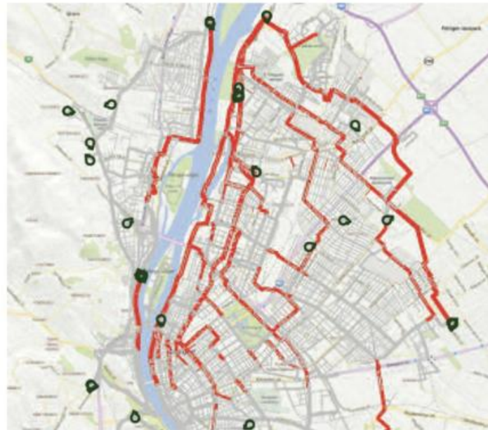
Figure 19 – Pipes sections in Budapest District marked in red where the minimum water speed exceeds 0.2 m/s in the main pipes
